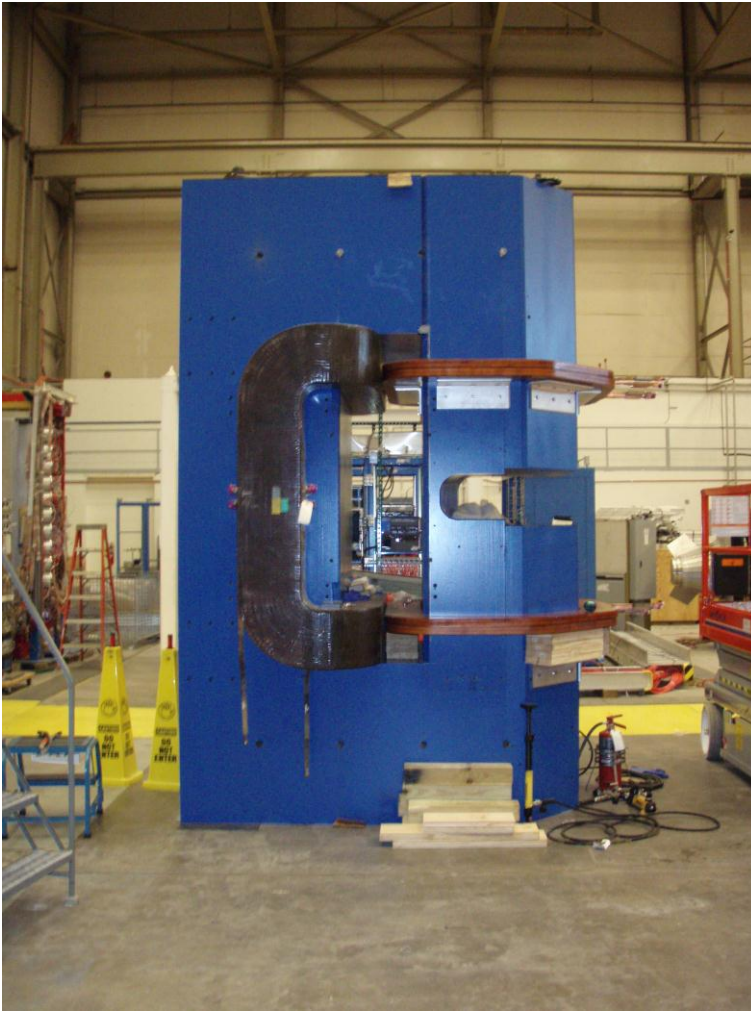
Figure 1 The SBS magnet assembled in the Testlab. The magnet will be tested with the original saddle coil and two of the racetrack coils. The beam cut out is on the right side. The cooling water and power are currently being connected for the low current ( 200A) test.
