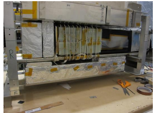
Figure 1: The left picture shows the 4x4 lead glass blocks with light guide and PMT. The right picture shows the heating element wrapped around the lead glass surrounded by glass foam bricks (enclosed in aluminum foil).
