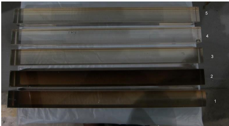
Figure 2: Lead glass blocks placed at various locations in the hall as a radiation monitor. The blocks labelled 1 and 2 were near the C16 and show significant darkening after the C16 was moved to 10°. The blocks labelled 3,4 and 5 were located at larger angles and show no darkening.
