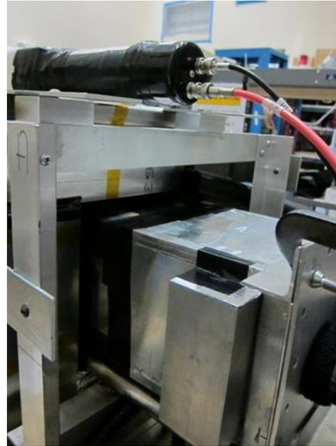
Figure 4 The left photo shows the back of the C16. Air was pumped from a blower into the back of the C16 to cool the PMTs down to about 38° C. The right photo is a close up of the light tight enclosure for the PMTs and bases.
