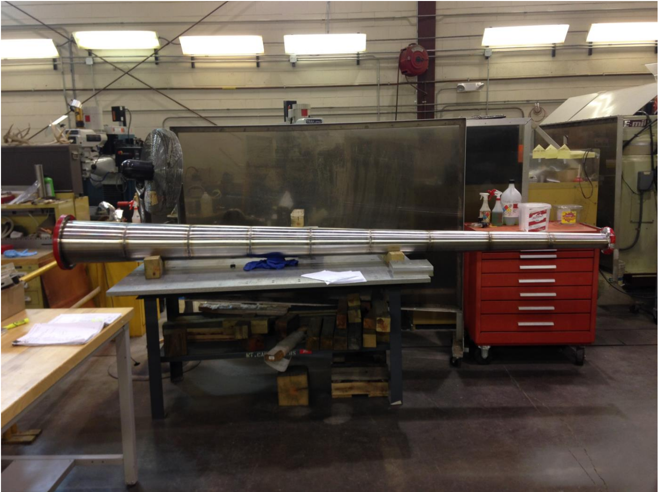
Figure 1 Completed vacuum pipe
