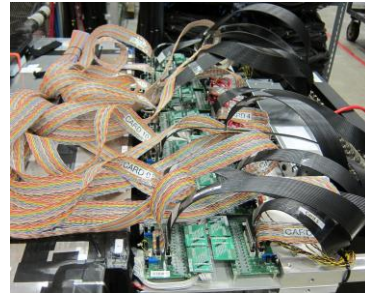
Figure 1 Left photo is the stack of CDet modules 2 and 3 which have been covered and enclosed. The right photo shows the electronics connected module 1 that is under going cosmic testing.
